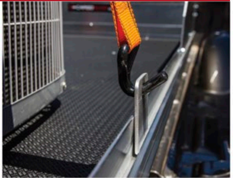
CGCLTD 4 - Outside Tie Downs
